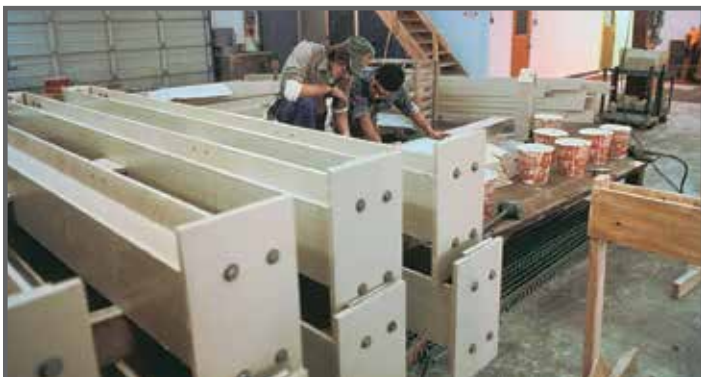
Fabricated Dynaform columns ready for shipment.
